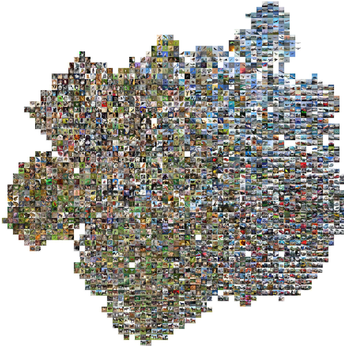
Figure 6.1: t-SNE visualisation of a subset of the CIFAR-10 image dataset (20,000 images). Image positions are computed using a 2-dimensional t-SNE projection (van der Maaten and Hinton (2008)) of a 32-dimensional embedding produced by the non-linear variant of my graph regularised projection function. Clusters of semantically related images are readily evident such as horses (bottom), airplanes (top right) and dogs (top left). Image best viewed in colour and ideally with a zoom tool on the electronic PDF version of the thesis.
